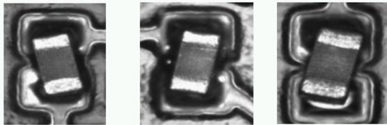
**Figure 5 – Angle Measurement by OGP AT8800, C99a at  $12.49^\circ$ (Left), C195a at  $10.73^\circ$  (Center), C226aat  $13.95^\circ$  (Right)**
