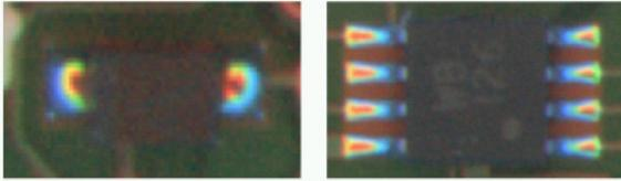
**Figure 3 - Polarity Mark on Black Diode and SOIC8**
