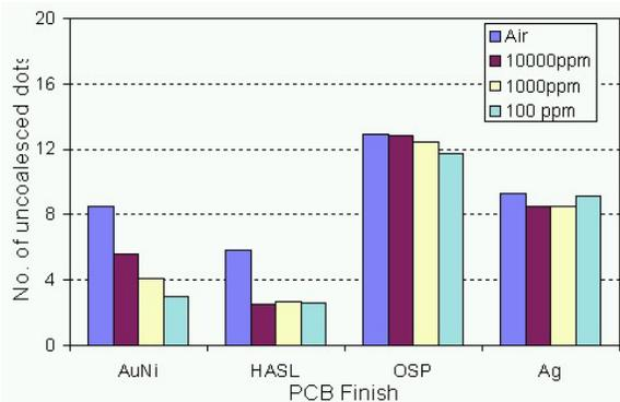
**Figure 17- Effect of Inerting on PCB Finishes**
