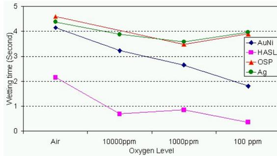
**Figure 10 - Wetting Time for PCB Finishes after 4 Reflows**
