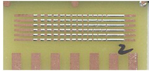
**Figure 4 - Test Coupon after Reflow with Paste**
