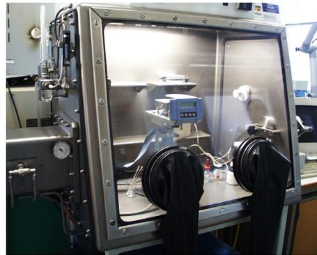
Figure 3 - Glove Box with Solderability Tester
