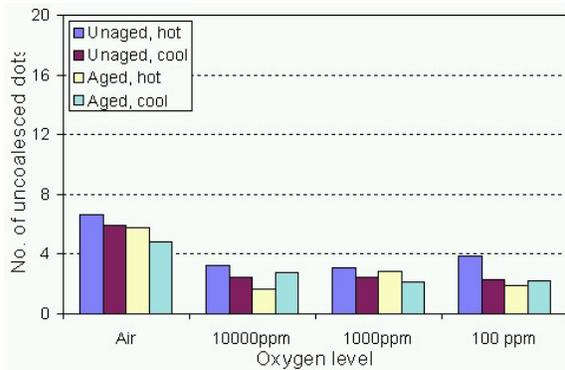
**Figure 13 - Spreading Measurements for HASL Finish, Averaged for Paste 1 and 2**
